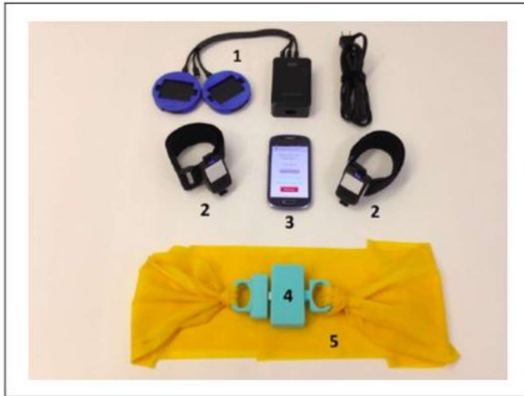
Figure 1. Components of a Rehabilitation-Internet-of-Things: wireless chargers for sensors (1), ankle accelerometers with gyroscopes (2) and Android phone (3) to monitor walking and cycling, and a force sensor (4) in line with a stretch band (5) to monitor resistance exercises.
